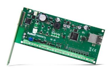
An Ethernet communicator is used in the PERFECTA-IP 32-WRL model. It allows you to use the mobile application, remote system configuration from the **PERFECTA Soft** program and event reporting (e.g. to a security agency monitoring station).
